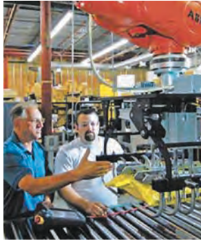
Heavy duty bag gripper shown lifting bags of rock salt off of conveyor during simulated product trials.
