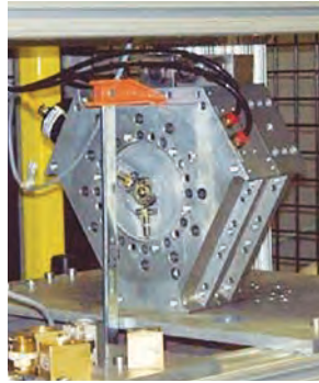
Cycle testing of piston and cam lock mechanism accomplished on a test stand which continuously couples and uncouples mating sides of Applied Robotics Tool Changers for literally millions of cycles.
