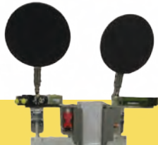
Cycle testing of piston and cam lock mechanism accomplished on a test stand which continuously couples and uncouples mating sides of Applied Robotics Tool Changers for literally millions of cycles.
